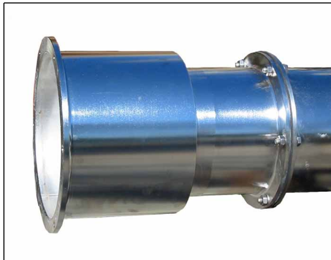
Figure 5: The Expansion chamber fitted to the barrel.
