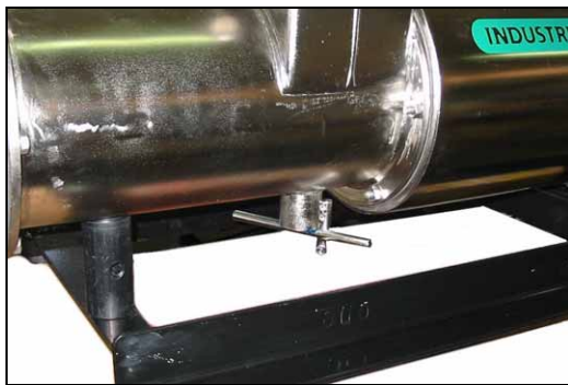
Figure 9 : Screen slot infill pin
