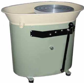
No.5 Cone drive potters wheel with hand operated speed lock
